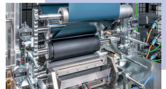
Open chamber doctor blade for small lacquer quantities
